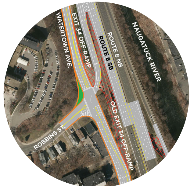
Relocated off-ramp to Robbins Street
