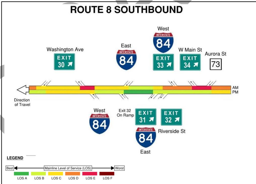
Figure 3-4. Route 8 Southbound Year 2045 Levels of Service, AM and PM Peak Hours, No-Build
