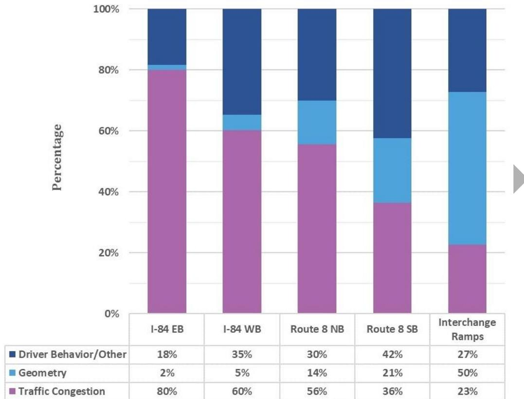
Figure 3-7. Mixmaster Interchange Crash Contributing Factors, 2015-2017
